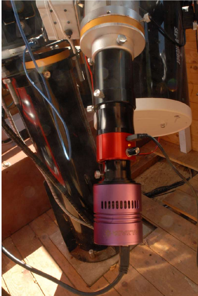
Daystar Quark filter on William Optics 110mm telescope making an effective F28 system
