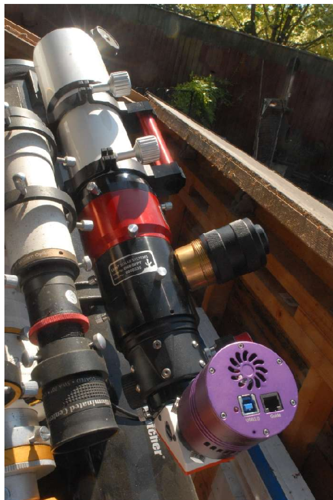
Lunt 80mm double stacked Ha modular telescope. Rotating the Etalons reduces reflected light.
