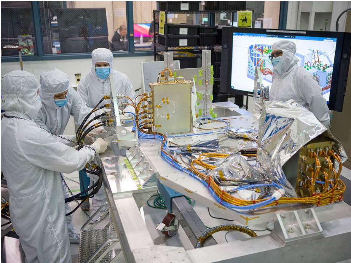
Engineers at NASA's Jet Propulsion Laboratory are shown assembling the electrical palette for the Coronagraph Instrument, which houses the electronics that receive instructions from the Roman spacecraft and send back the Coronagraph Instrument's scientific data.
