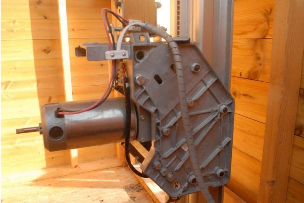
Motor for top section (the hex rod allows for manual operation in an emergency, either by hand or battery drill)
