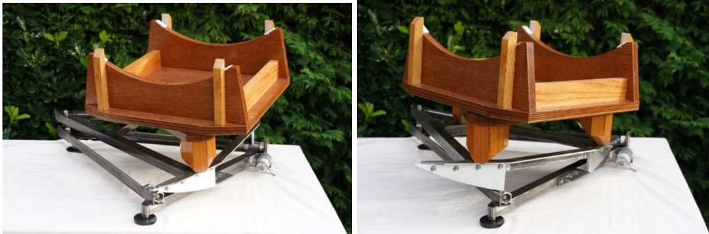
Two views demonstrating the angular movement for approximately 60 minutes, shown with telescope ground board and rocker box on top.
