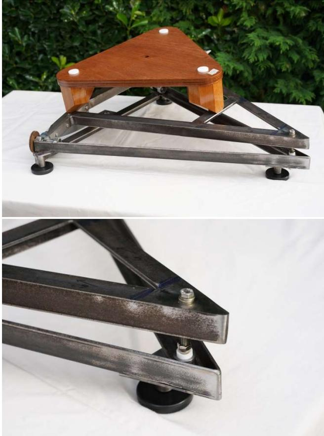
The platform is aligned north south, the point of the triangular frame faces south and the pivot point called the south bearing.
