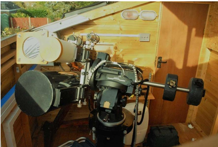
The image shows the general arrangement (set up for white light solar imaging.) The ETX125 with solar filter is on the auxiliary mount. Above the William Optics is a homemade solar finder with a 50mm William Optics finder behind. On the wall by the door (below the red and white lights) is the second control panel for the roof.
